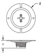
Material: High Density Polyethylene (HDPE), Steel
