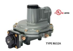
Type R632A has 1/8 in. NPT built-in gauge taps orificed to a No. 54 drill size, on the upstream and downstream sides. These taps provide easy access for testing the proper operation of the First and Second-Stage while the system is pressurized. This regulator also features a large 3/4 in. drip-lip vent to reduce the chance of blockage by freezing rain or sleet when properly installed with the vent pointing down.
