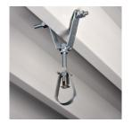
The 115M Standard Duty Loop Hanger is ideal for suspending stationary, non-insulated pipe lines, including CPVC pipes, in fire sprinkler systems. A knurled insert nut helps simplify vertical adjustments and flared edges on the base (1/2" to 4" sizes) help protect pipes from coming into contact with any sharp edges of the hanger.
