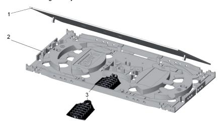
Overview Optical Fibre Splice Cassette 1=lid, 2=splice cassette, 3=splice protector holder 6-way
