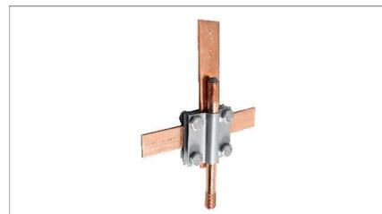
Cruciform clamp – profile, bolted M8 with stainless steel separator, to connect rod to galvanized tape or circular conductor (with stainless steel separator inside protecting from corrosion between copper and zinc when different metals are connected)
