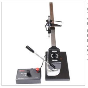
These loaders allow torque wrenches to be calibrated or tested in accordance with ISO 6789:2003, BS EN 26789:2003 and American military standard GGG-W-686. Their function is to take full advantage of the accuracy of Norbar's torque measuring systems by reducing operator induced variations in the calibration process.
