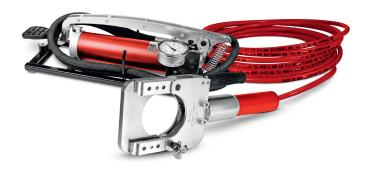
Safety hydraulic cable cutting set for Al and Cu cables, when the voltage is impossible to determine. Equipped with hydraulic head, pump with manometer and automatic retraction, earthing wire, hydraulic hose (10 m). Maximum nominal tension – 60 kV.
