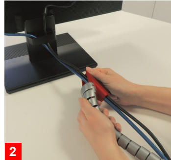
2 Insert the pointed part of the tool into the end of the sheath.
