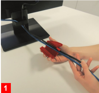
1 Cut the sheath to the desired length. Gather all cables into the tool. Close the tool.
